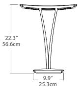
Aradess Table Lamp Model No. ARD-22T-PC (Polished Chrome) Fixture Wattage:22W Approx. fixture output: 1435 Lm
